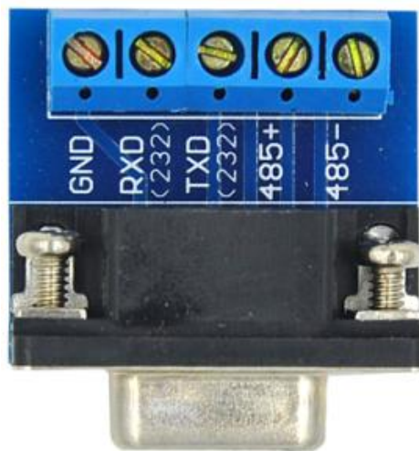
Chart 4 DB9To the terminal adapter plate
