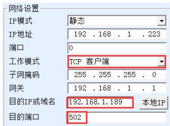
Chart 17 Modbus TCP being client side
